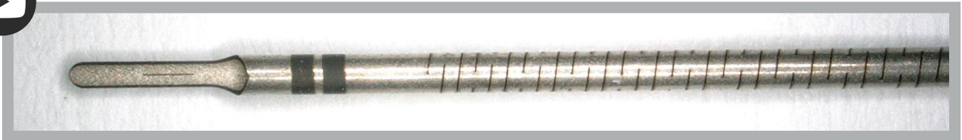
Figure 1. Hypotube sample made with a Coherent StarCut Tube Hybrid. The outer diameter is 0.7 mm.
