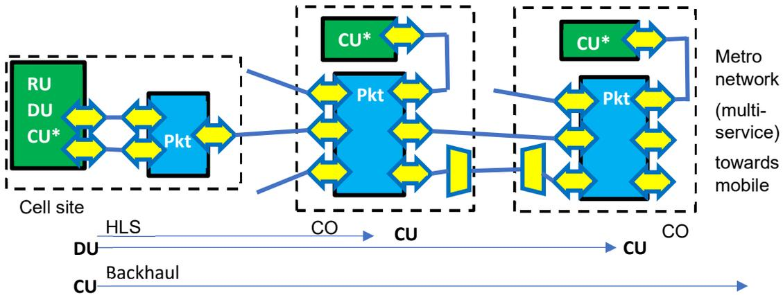
Figure 20: Backhaul and HLS for DRAN and virtual RAN. CU\* indicates possible locations for the CU, at the cell site, or at the closest CO. The latter constitutes the VRAN case. The pluggables at the CO sites may be C-temp as indicated by dashed borders for the intraoffice ones.
