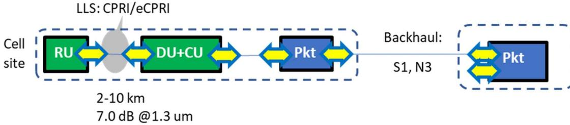
Figure 11: 10 km RU-DU direct parallel fibers Blueprint.
