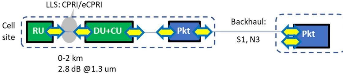
Figure 10: 2 km RU-DU direct parallel fibers Blueprint.
