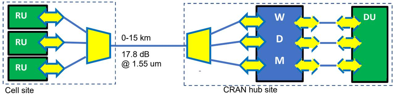
Figure 17: 15 km RU-DU semi-active wavelength multiplexed, P2P or P2MP Blueprint. The intraoffice pluggables at the hub site may be C-temp as indicated by dashed borders.
