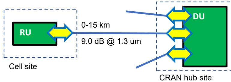
Figure 13: 15 km RU-DU direct parallel fibers Blueprint.
