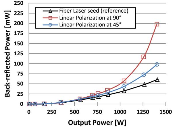
Figure 3: Back-reflected power vs. amplifier output power for 90° and 45° output linear polarization.
