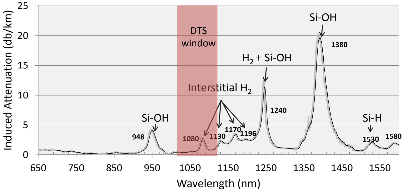
High temperature and hydrogen environments induce losses
