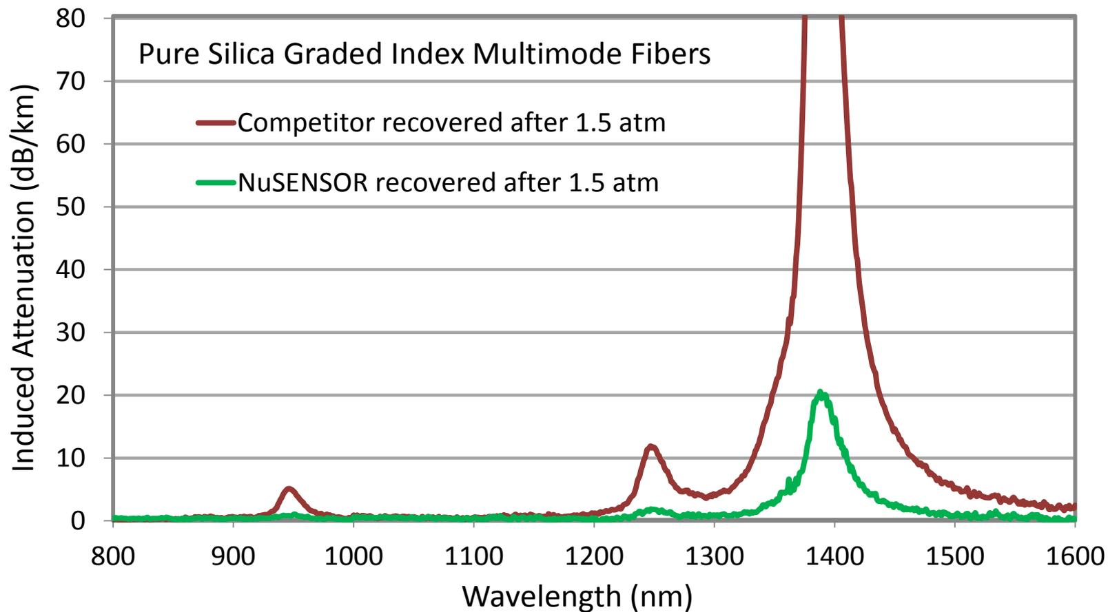
Significant differences in hydrogen induced-attenuation can be observed in nominally pure silica fibers due to processing differences
