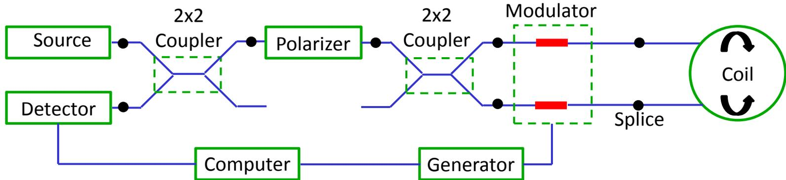
Counter rotating waves traveling through the same circular path exhibit a phase difference
