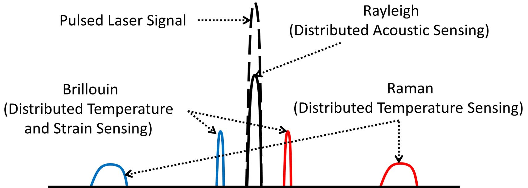
Fiber serves as a continuous sensing element. Sensing is based on
