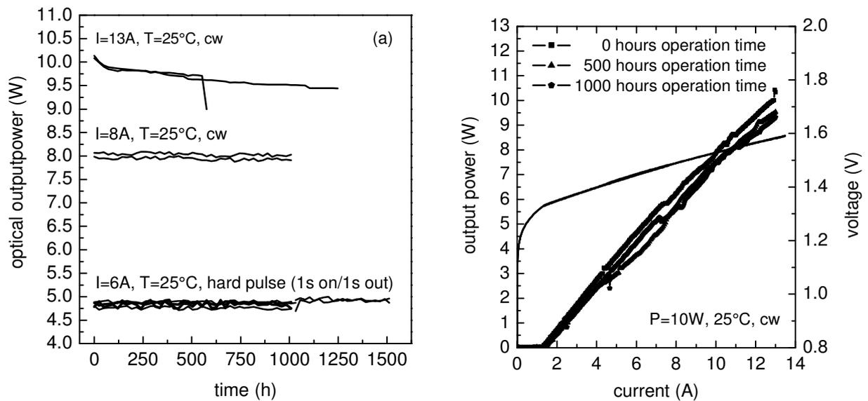
Figure 9: (a) Lifetime measurements of tapered lasers at 6A, 8A and 13A operation current and 25°C heat sink temperature. (b) On the right hand side P-I-curves of one tapered laser operated at 10W after different operation times.
