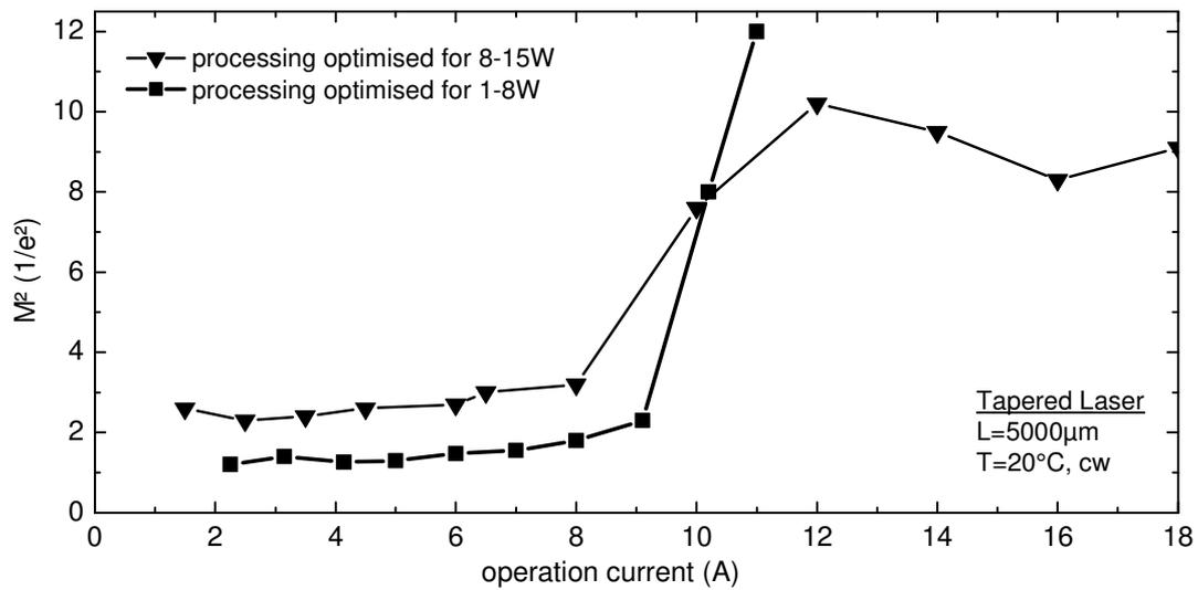
Figure 4: Measurement of the beam quality parameter M² for two tapered lasers optimized in etching depth for optimal beam quality below 8W and between 8W and 15W. All measurements have been performed at 20°C heat sink temperature in cw operation.
