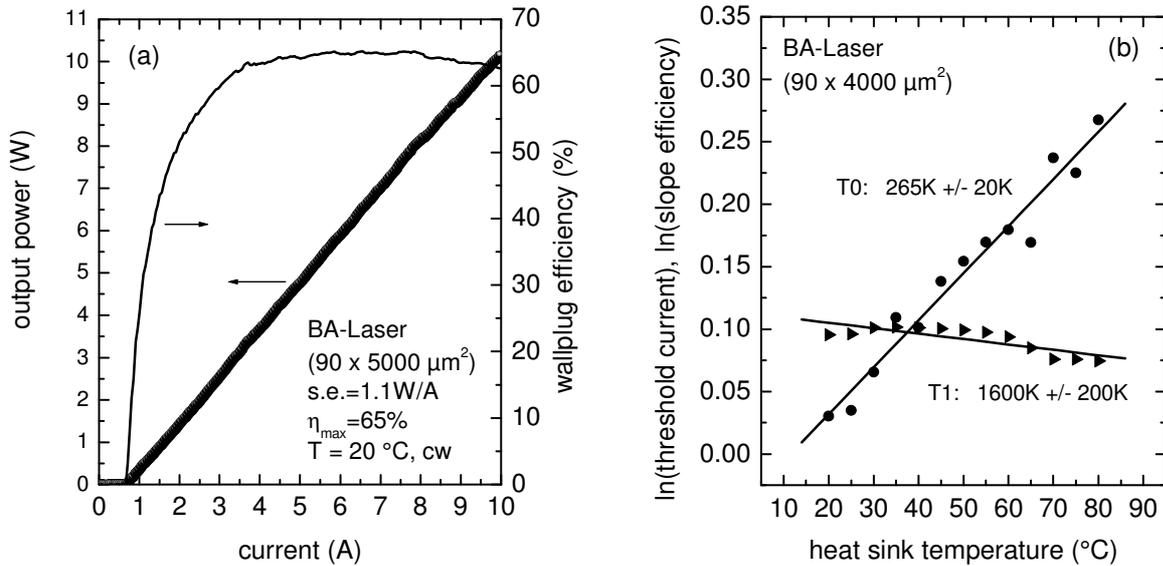
Figure 2: (a) P-I-curve of a BA-laser in  $(100 \times 5000 \mu\text{m}^2)$  geometry at 20°C heat sink temperature. (b) P-I-curves of a BA-laser in  $(100 \times 4000 \mu\text{m}^2)$  geometry at different heat sink temperatures. All measurements have been performed in continuous wave operation.
