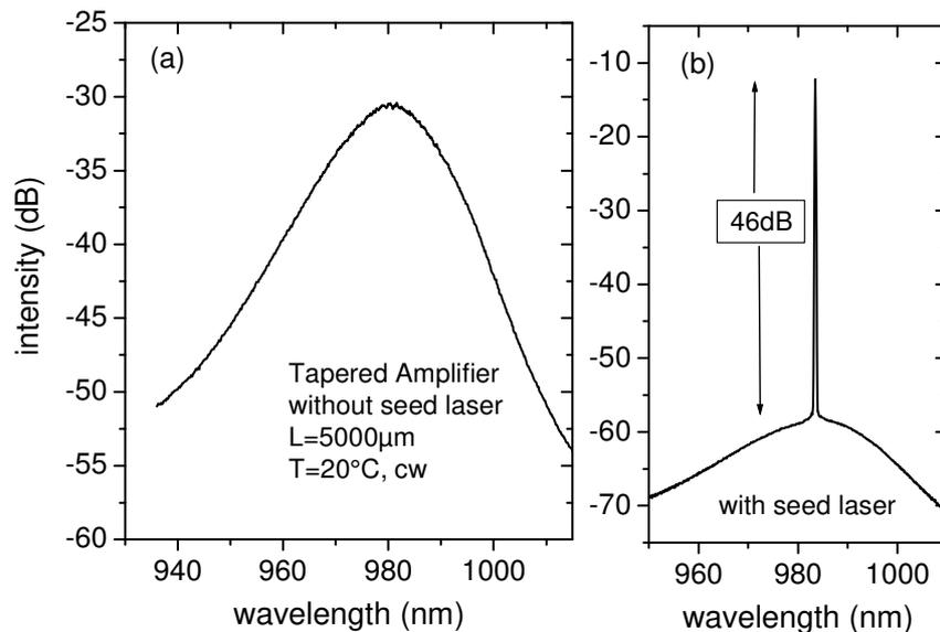
Figure 6: a) free running spectra without seed laser of tapered amplifiers at 976nm with 5mm overall resonator length. b) Spectrum of a tapered amplifier within a MOPA configuration. The measurements have been done at a heat sink temperature of 20 °C in cw operation.
