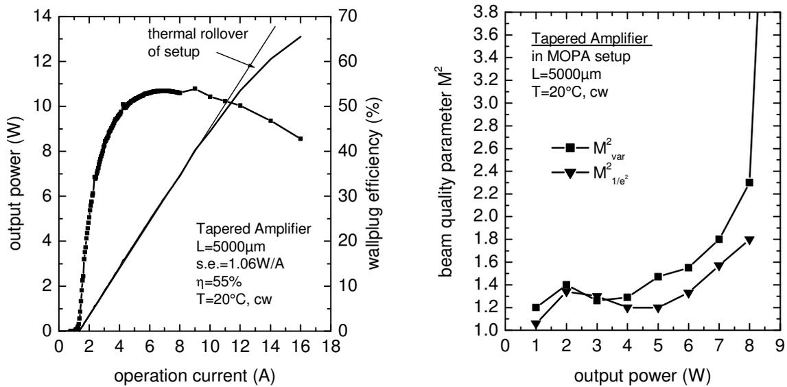
Figure 5: (a) P-I-curve of a tapered amplifier with 5mm overall resonator length in a MOPA setup with 20mW seed power. (b) Measurement of beam quality parameter M2 in dependence of output power. All measurements have been performed at 20°C heat sink temperature in cw operation.
