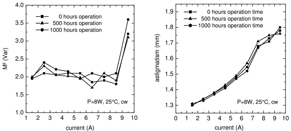
Figure 10:  $M^2$  and astigmatism of a tapered laser operated at 8W in the lifetime test of figure 9a in dependence on operation current after different operation times.
