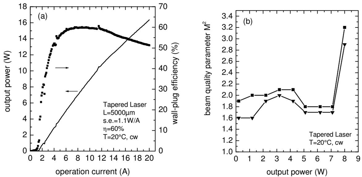
Figure 3: (a) P-I-curve of a tapered laser with 5mm overall resonator length. (b) Measurement of beam quality parameter M2 in dependence of output power. All measurements have been performed at 20°C heat sink temperature in cw operation.
