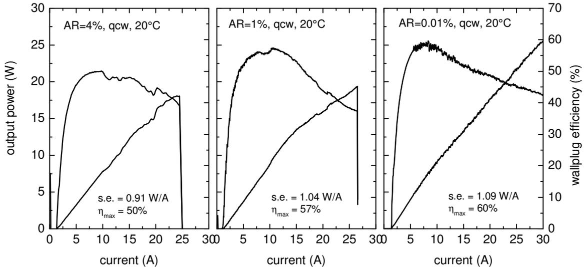
Figure 8: COMD measurements of 5mm long tapered lasers with different front facet coatings. All measurements have been performed at 20°C heat sink temperature at a pulse time of 50 $\mu$ s and a repetition rate of 50Hz.
