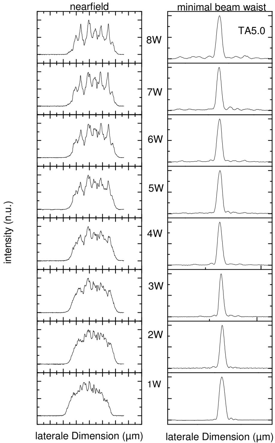
Figure 7: Beam profiles of a 5mm long tapered amplifier in MOPA configuration at the front facet (near field) and at the minimal beam waist in dependence on different output powers.
