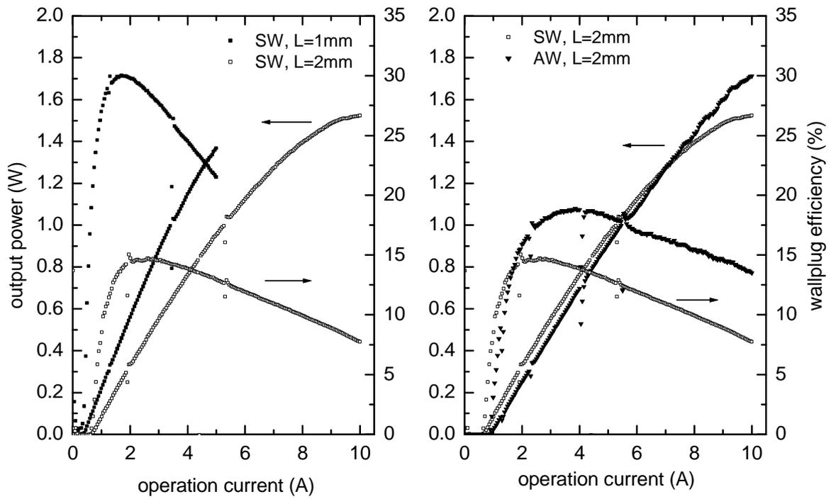
Fig. 7. (a) Electro-optical characterisation of SW diode lasers with 1mm and 2mm long resonators. (b) Electro-optical characterisation of SW and AW diode lasers with 2mm resonator length. All measurements have been done in cw operation at  $20^\circ\text{C}$  heat sink temperature.
