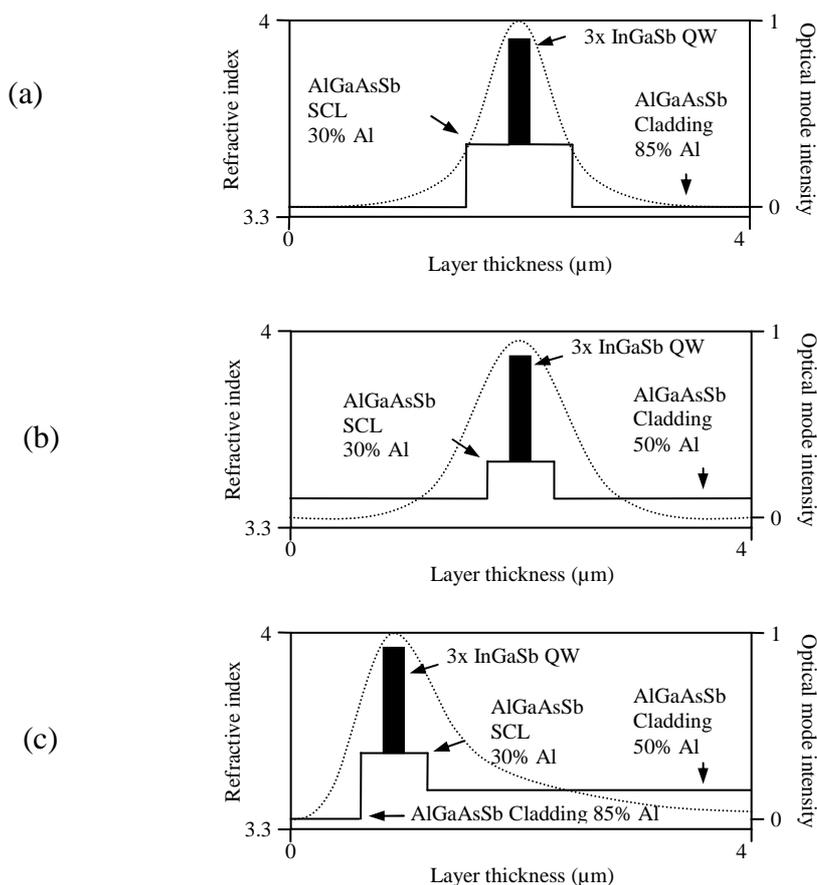
Fig. 2 (a) Schematic refractive index profile (left scale) and calculated optical mode intensity (right scale) of a conventional broadened waveguide design. (b) Schematic refractive index profile (left scale) and calculated optical mode intensity (right scale) of a narrow waveguide structure. (c) Schematic refractive index profile (left scale) and calculated optical mode intensity (right scale) of an asymmetric waveguide.
