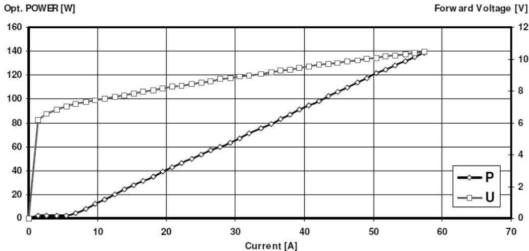
Figure 12. CW output power vs. current characteristics for a 10-bar-stack at 1908nm. All measurements have been performed at 20°C heat sink temperature in cw mode.
