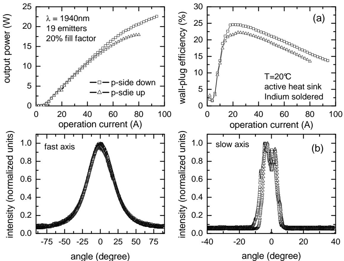
Figure 8. a) CW output power vs. current characteristics for 20% fill-factor bars emitting at  $1.94\mu\text{m}$ . The bars have been packaged by Indium soldering on actively cooled heat sinks either in p-side up or down mounting. b) Corresponding far field measurements at  $40\text{A}$  cw operation in slow- and fast-axis direction. All measurements have been done at  $20^\circ\text{C}$  heat sink temperature.
