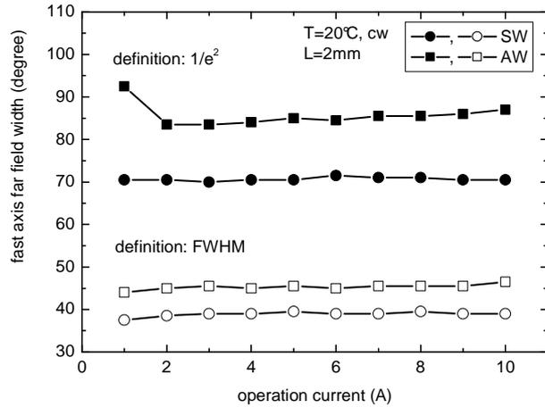
Fig. 6. Fast axis far field widths for SW and AW lasers at  $1.94\mu\text{m}$  with 2mm resonator length. All measurements have been done in cw mode at  $20^\circ\text{C}$  heat sink temperature.
