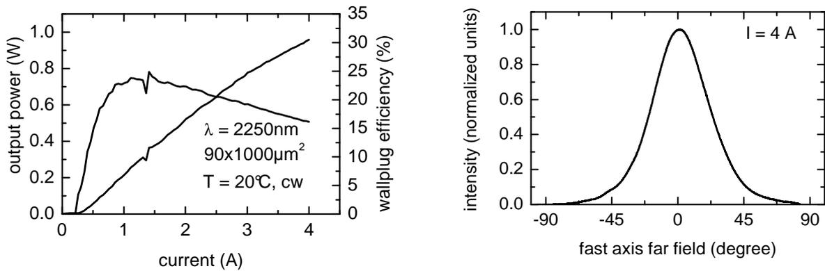
Figure 4. Output power-vs.-current characteristics and current dependent wall-plug efficiency of a broad-area single emitter at 2.25 $\mu\text{m}$  with narrow waveguide structure (left hand-side). Corresponding fast axis far field at 4A (right hand-side). The measurements have been carried out at a heat sink temperature of 20  $^{\circ}\text{C}$  in continuous wave mode (cw).
