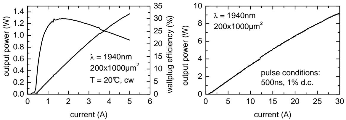
Figure 3. Output power-vs.-current characteristics and current dependent wall-plug efficiency of a broad-area single emitter at 1.94 $\mu\text{m}$  with narrow waveguide structure. The measurements have been carried out at a heat sink temperature of 20  $^{\circ}\text{C}$  in continuous wave mode (cw) (left hand-side) and in pulsed mode (right hand-side, 500ns, 1% d.c.).
