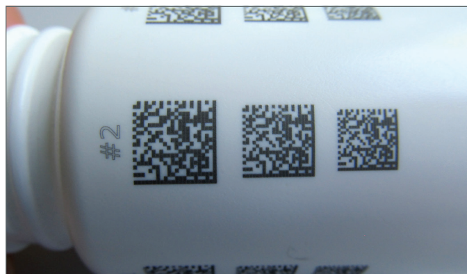
Figure 3. Ultraviolet laser marking is ideal for QR codes on plastic bottles and packages including HDPE.
