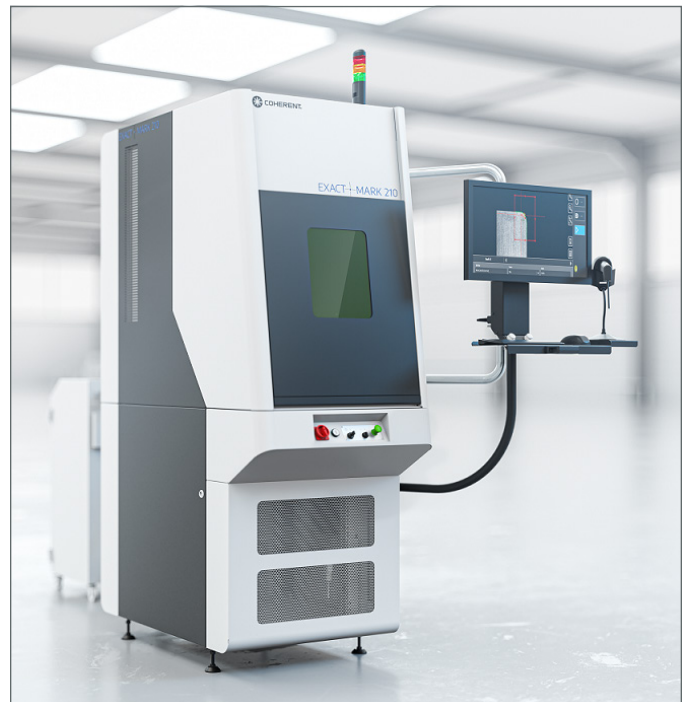
Figure 2. A small footprint and object-driven touchscreen control maximize the value and utility of the ExactMark 210.
