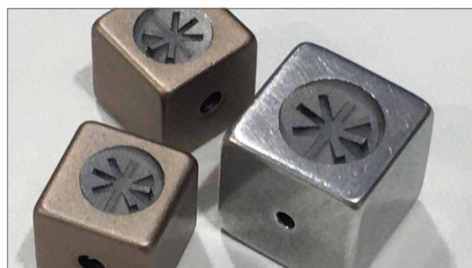
Figure 3: The same EasyMark can also create deep 3D engraving.
