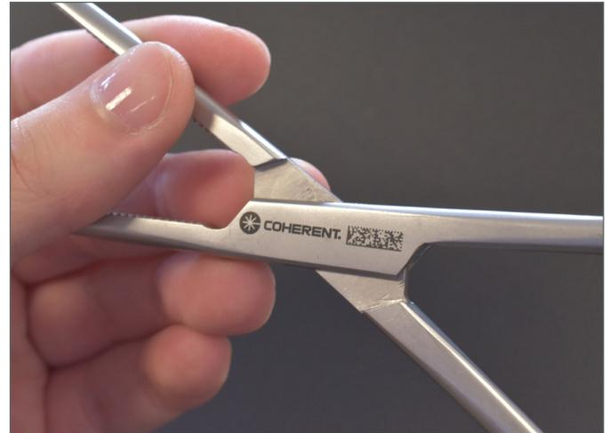
Figure 1. Laser black marking produces a high-contrast mark on metal surfaces with enhanced corrosion resistance.
