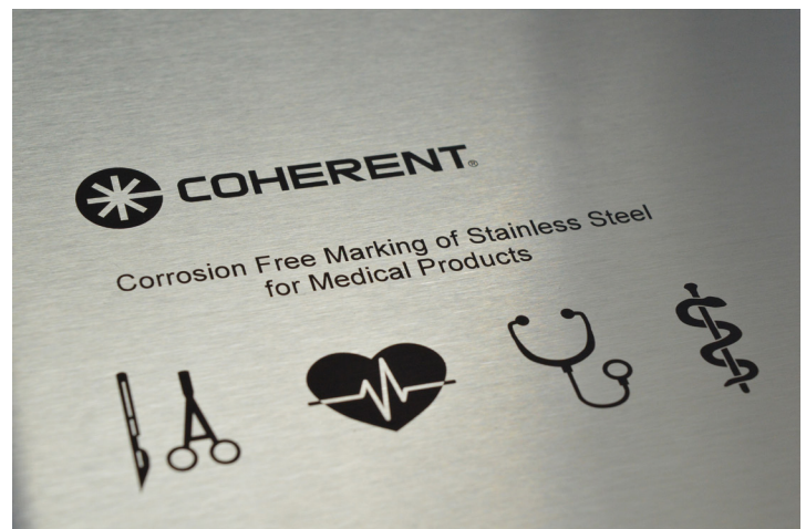
Figure 3. Black marking creates high contrast marks on steel and aluminum surfaces without affecting surface anodization or passivation.
