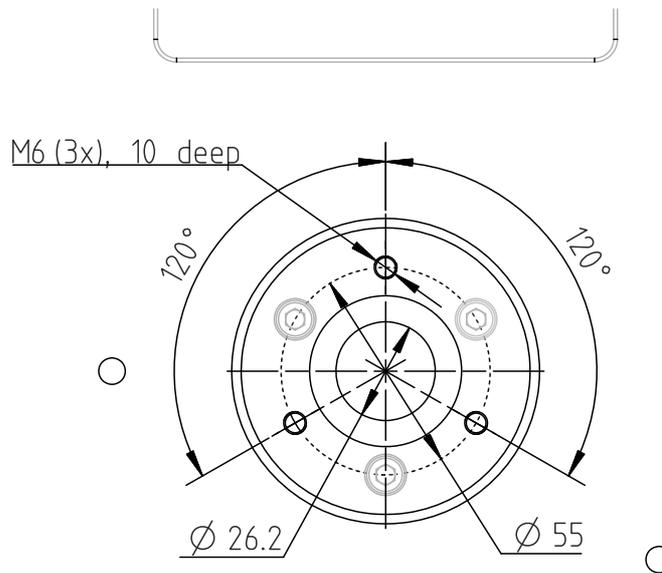
**Figure 8:** Mechanical interface at the beam exit aperture
