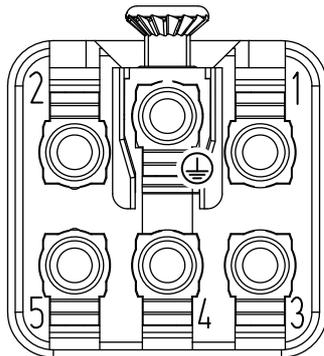
**Figure 18:** HAN Q5/0 Quick Lock female connector
