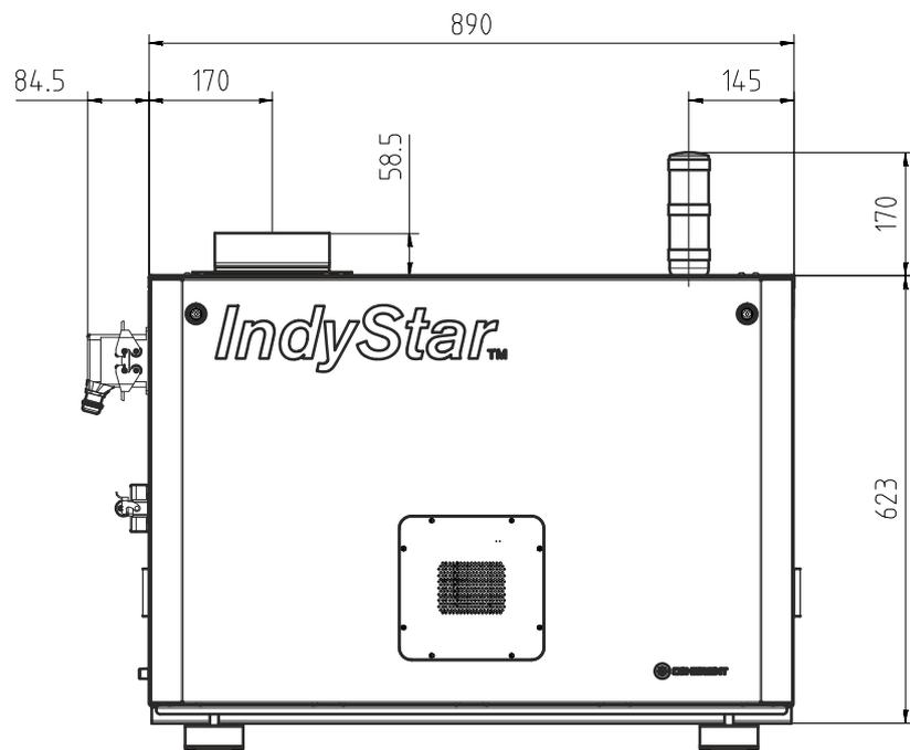
Figure 1: Dimensions, right side view
