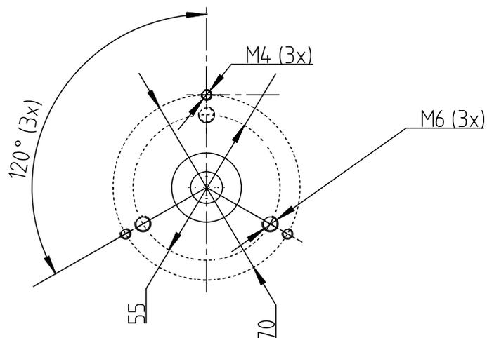
**Figure 10:** Threaded holes at diagnostic beam exit aperture
