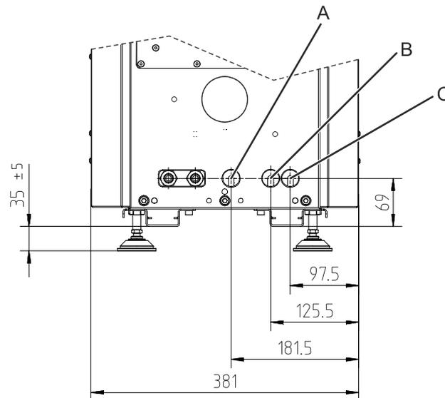
**Figure 16:** Gas connections
