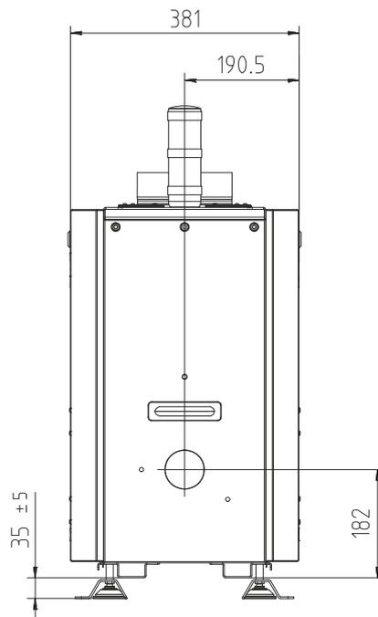
**Figure 4:** Dimensions, beam exit side view
