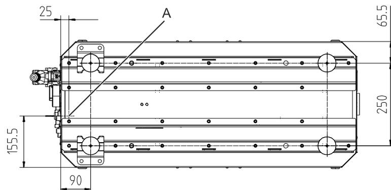
**Figure 20:** Position of water drainage outlet
