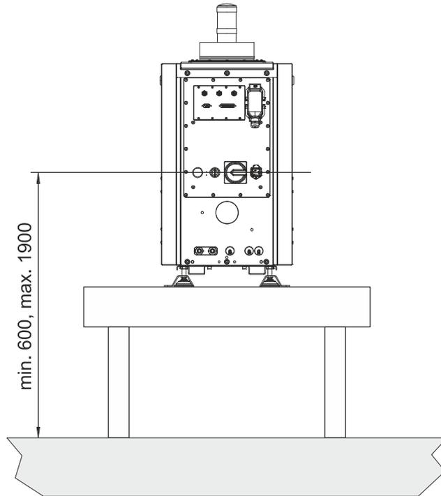
**Figure 13:** Required mains switch position
