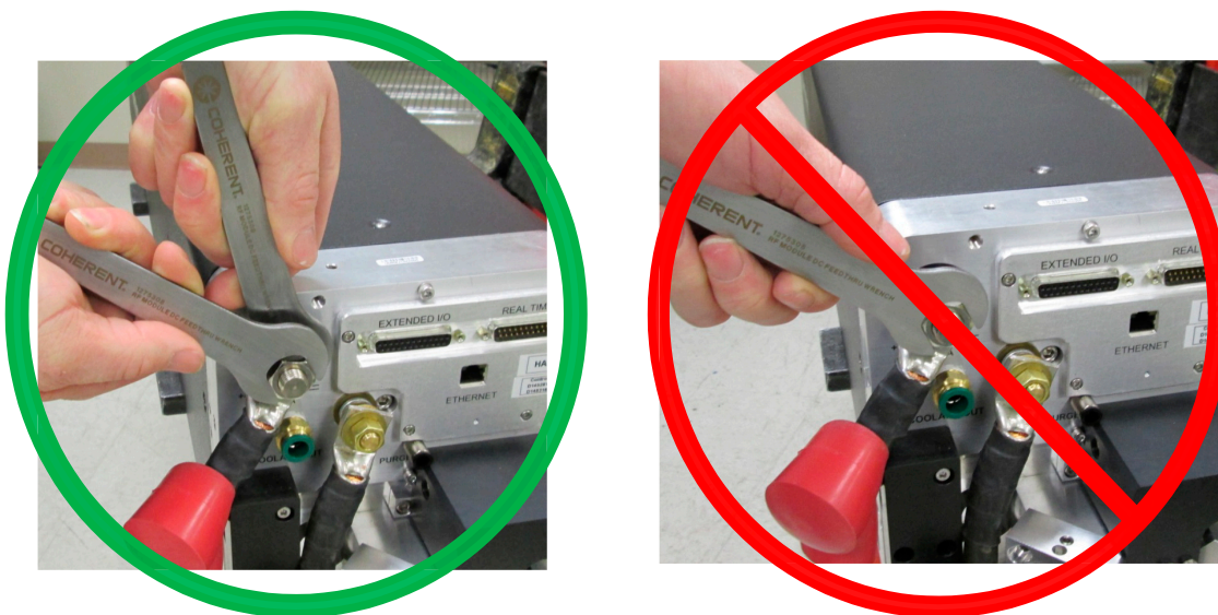
Figure 4-17. +48 VDC Location and Using Two Wrenches
