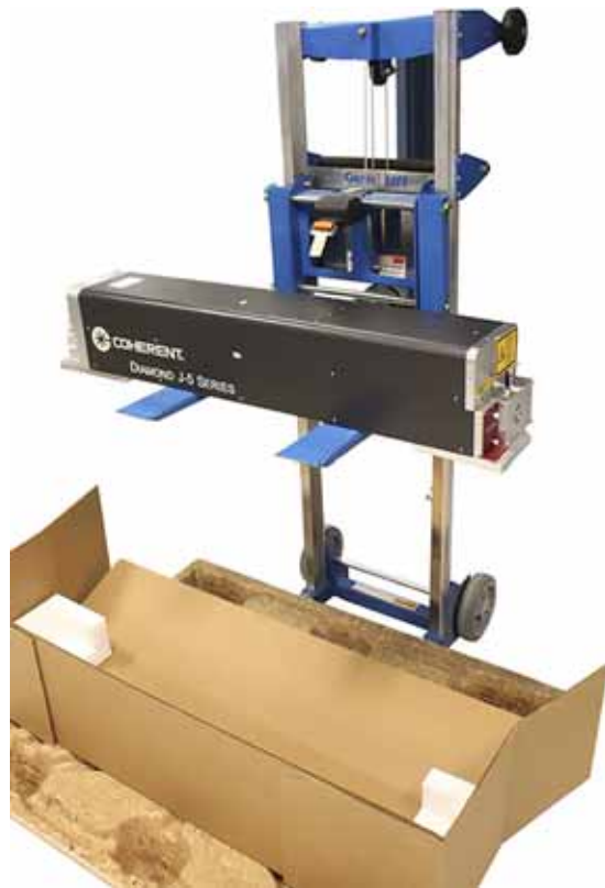
Figure 4-9. Lifting the Laser (J-2 and J-5 Series lasers shown as examples)
