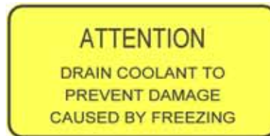
7 – Drainage Warning Label
