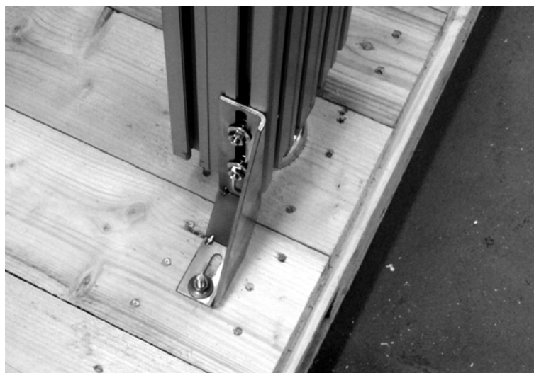
Figure 21: Main frame secured on base pallet
