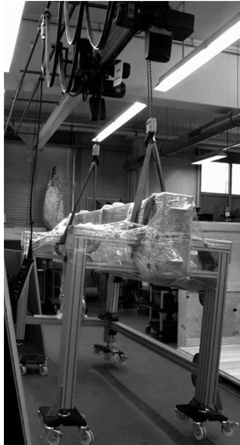
Figure 26: Lifting the main frame with a crane
