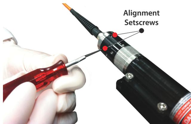
**Figure 4-61. Adjust the Fiber Ferrule**
