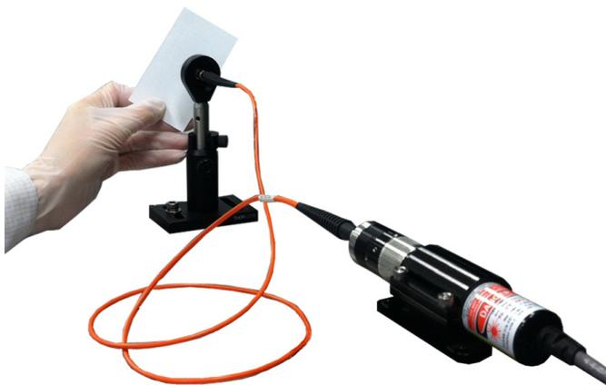
**Figure 4-60. Align White Target**
