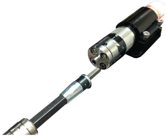
**Figure 4-67. Torque the Set Screws**
