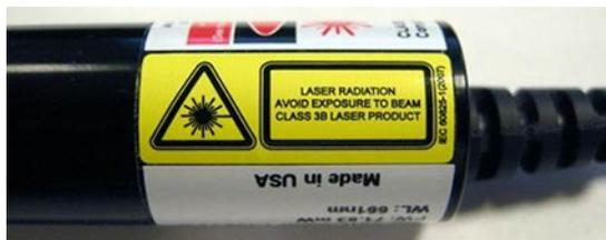
Figure I-2. Example of Safety Labels Wrapped on Laser
