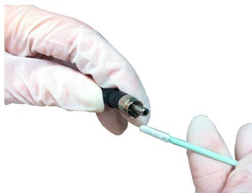
**Figure 4-58. Clean the Connector Ferrule**
