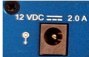
**Figure 3-11. Power-In Connector – StingRay/BioRay Remote**
