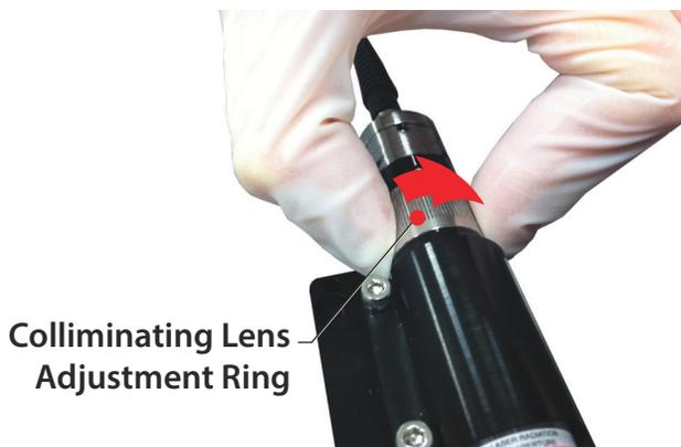
Figure 4-64. Adjust the Collimating Lens
