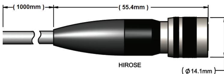
**Figure 8-118. Dimensions - Hirose Connector**
