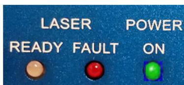
**Figure 6-95. LEDs on the Remote**
