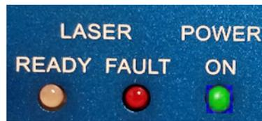
**Figure 3-8. LEDs on the Remote Front Panel**
