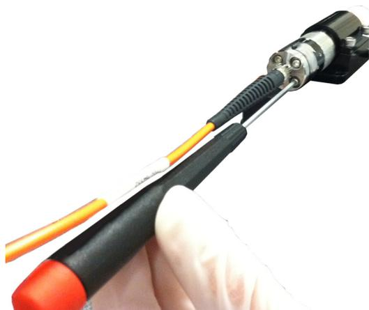
Figure 4-65. Tighten FR Adapter Assembly
