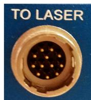
**Figure 3-13. Hirose Connector to Laser**
