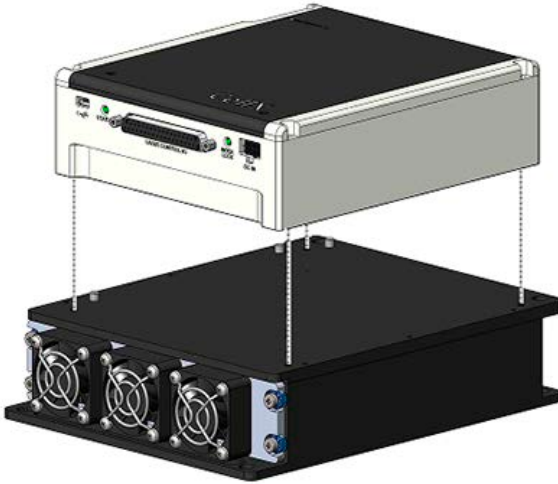
Figure 6. CellX on the Fan-Cooled Heat Sink
