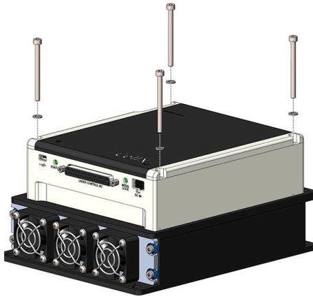
Figure 7. Align Washers and Screws in Both Units
