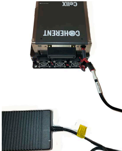
Figure 19. Connect Power Supply to Heat Sink Extension
