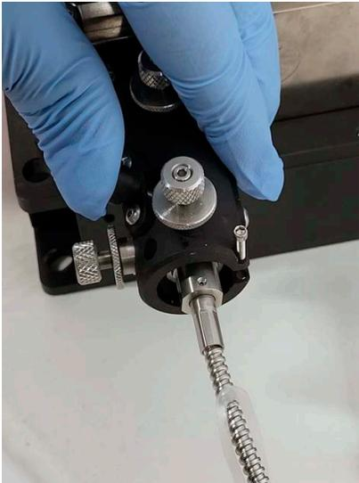
**Figure 8-16. Fiber Launcher with Fiber Installed**
