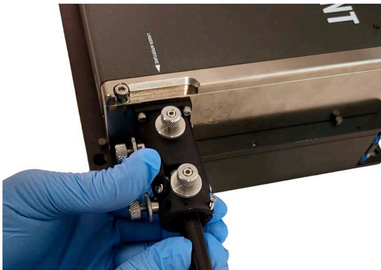
**Figure 8-40. Push Release/Hold Button and Remove Alignment Tube**
