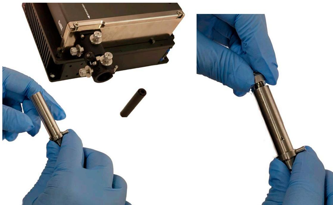
**Figure 8-33. Remove Fiber From Launcher and Install Cap**
