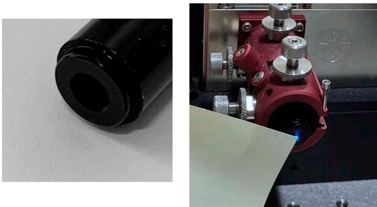
**Figure 8-39. Beam Aligned in Center of Alignment Tool/Aperture**
