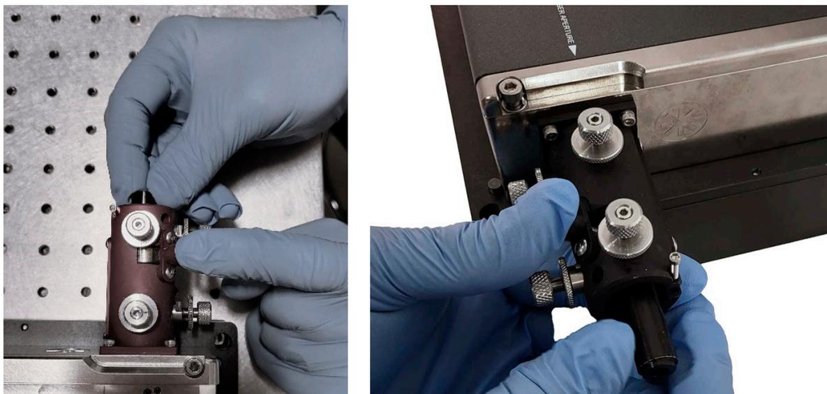
**Figure 4-35. Remove Alignment Tool**
