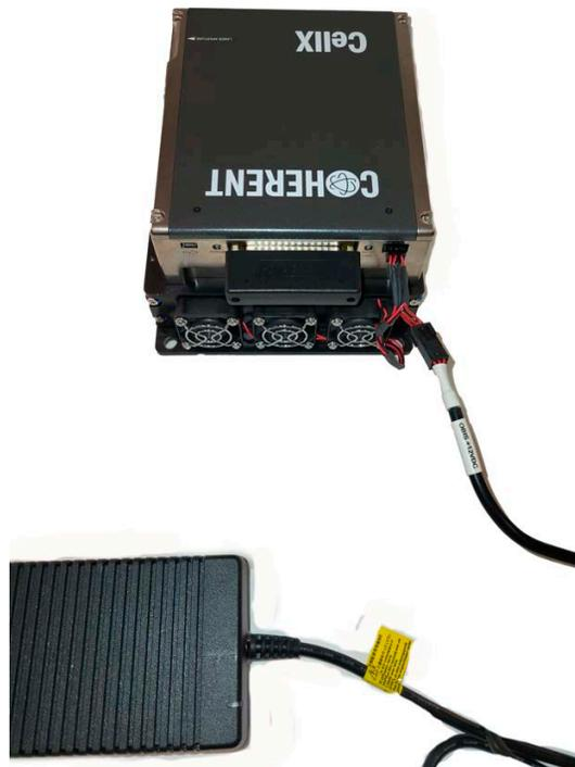
**Figure 4-27. Connect Power Supply to Heat Sink Extension**
