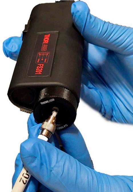
Figure 8-47. Put Fiber in FC Adapter
