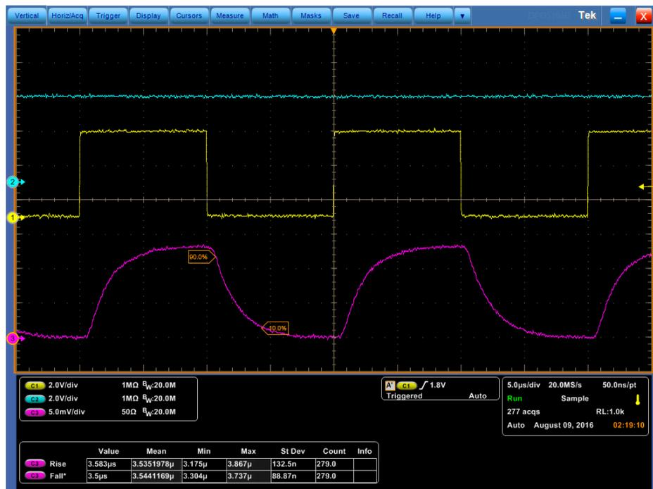
**Figure 5-8. Analog Modulation–LX 405 nm Laser @ 50 KHz**
