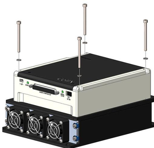
**Figure 4-4. Align and Set Washers and Screws in Both Units**
