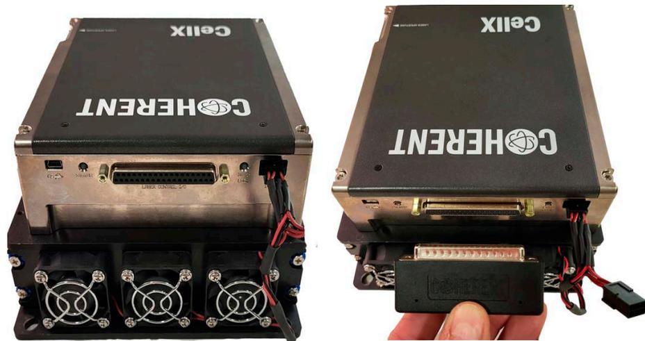
**Figure 4-9. Laser Control I/O Port on CellX and Interlock Plug**
