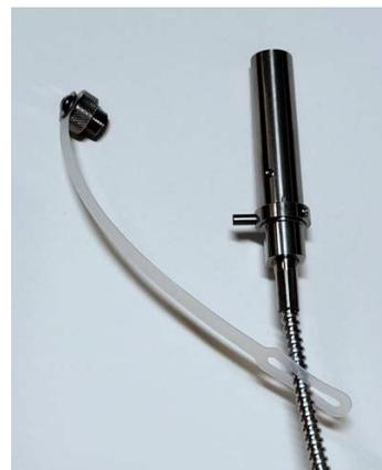
**Figure 4-40. Protective Cap Removed**
