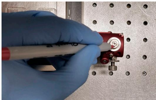
**Figure 8-37. Temporary Location Marking**
