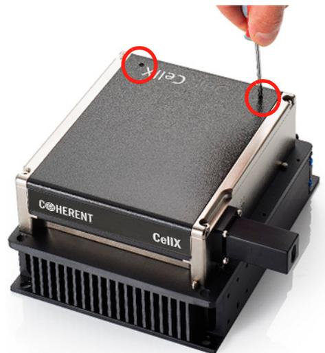
**Figure 8-14. Reinstall the Top Cover**
