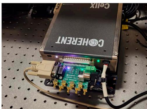
**Figure 4-13. RS-232 Connection from Control Board on a CellX**
