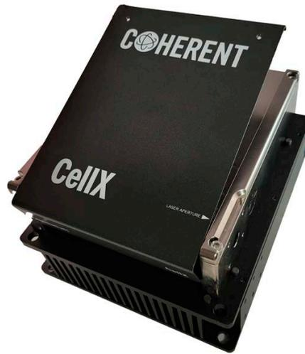
**Figure 8-3. Remove Top Cover off of CellIX**
