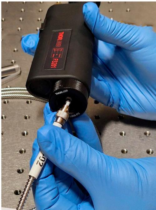
**Figure 4-39. Attach Fiber to Scope (FC example)**
