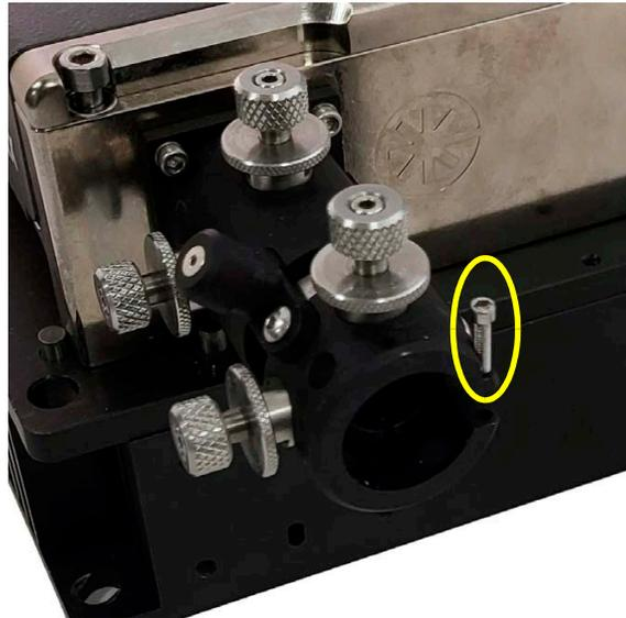
**Figure 4-37. Fiber Hold-down Screw Location**
