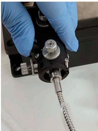
**Figure 4-43. Fiber Completely Inserted**
