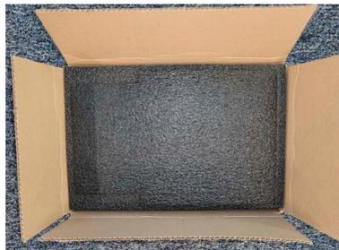
**Figure 11-5. Top ESD Foam Layer in Place**
