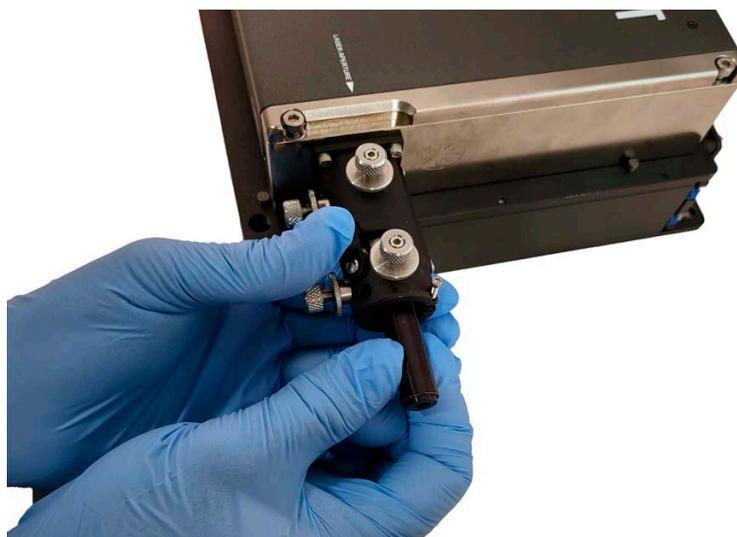
**Figure 8-43. Remove Alignment Tool/Tube**
