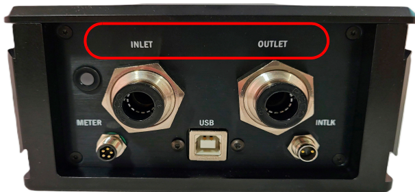
Figure 14. Water Inlet and Outlet Fitting Labels
