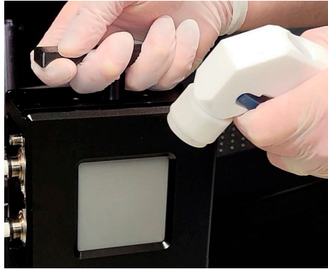
Figure 3. Use Clean Dry Air to Remove Dirty Material
