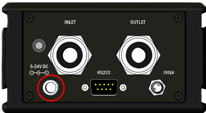
Figure 23. Power Connector - PM10K+ RS-232 Model
