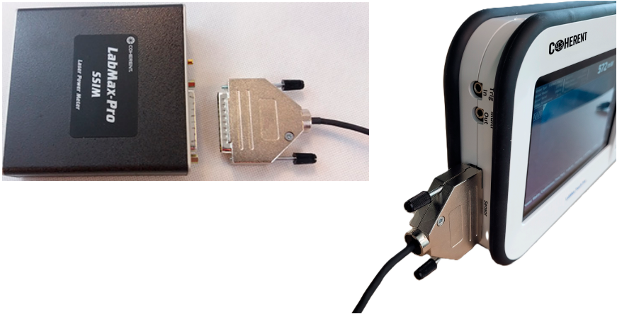
Figure 22. Connect Sensor to Meter with DB25 Cable
