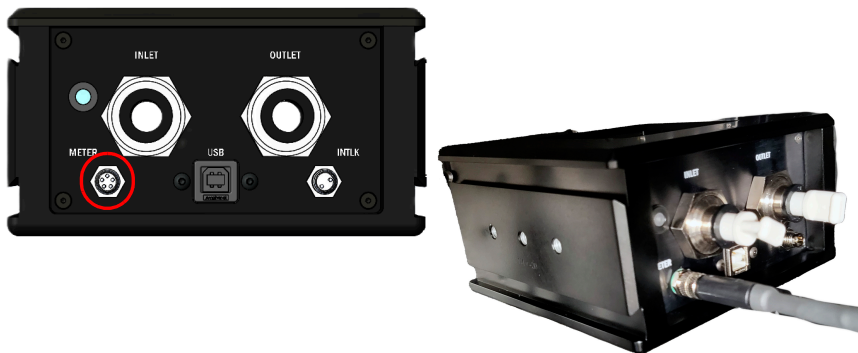
Figure 21. Meter Cable Connector - USB + DB25 Model Example
