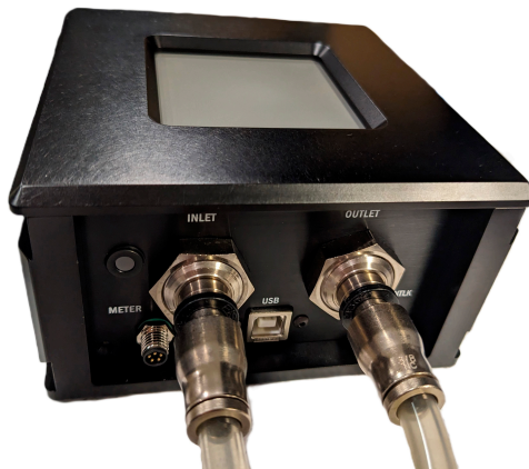
Figure 17. Water Hoses Installed With Step-down Fittings
