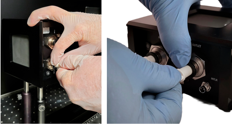
Figure 13. Remove Protective Caps
