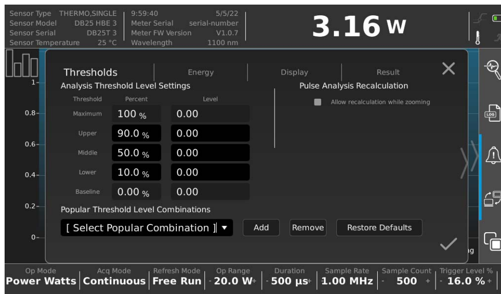
Figure 4-25. Pulse Analysis - Thresholds
