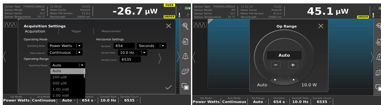
Figure 5-15. Auto Range Mode Selection - via Settings Menu or via Bottom Button Panel
