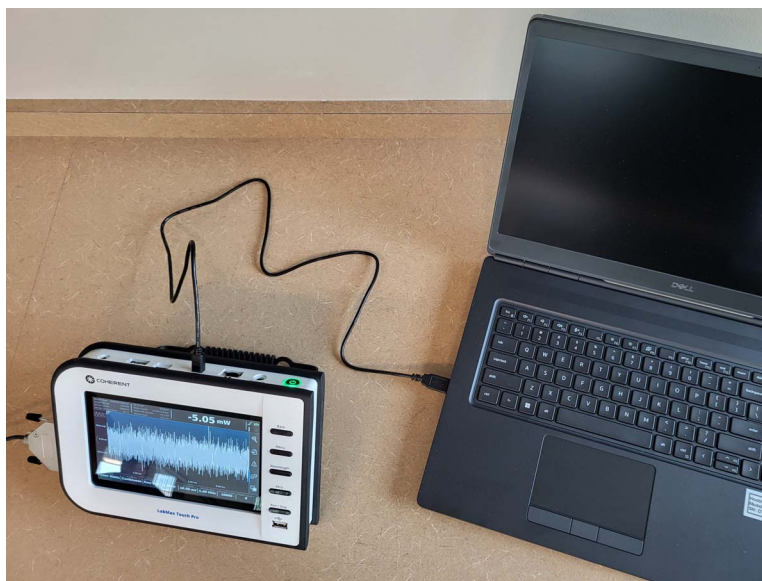
Figure 3-4. Connect the Meter to a PC
