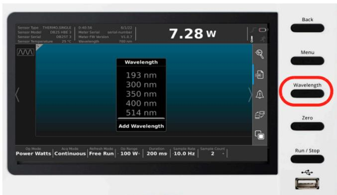
Figure 13. WAVELENGTH and ZERO Function Buttons
