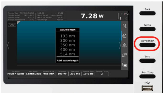
Figure 17. WAVELENGTH and ZERO Function Buttons
