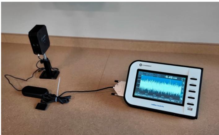
**Figure 10. Connect the Meter to a Sensor**
