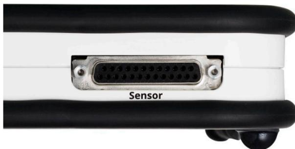
**Figure 3. 25-pin connector**
