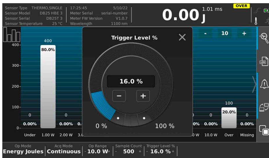
Figure 5-23. Trigger Level Setting
