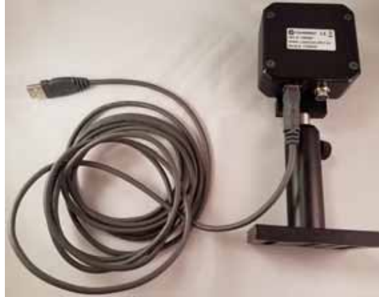
Figure 3-1. Connect USB Cable to Camera
