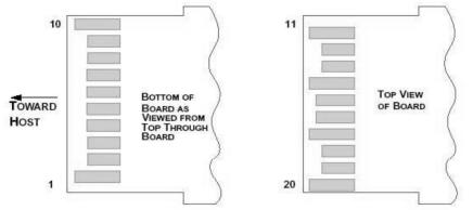
Figure 1. Diagram of Host Board Connector Block Pin Numbers and Names
