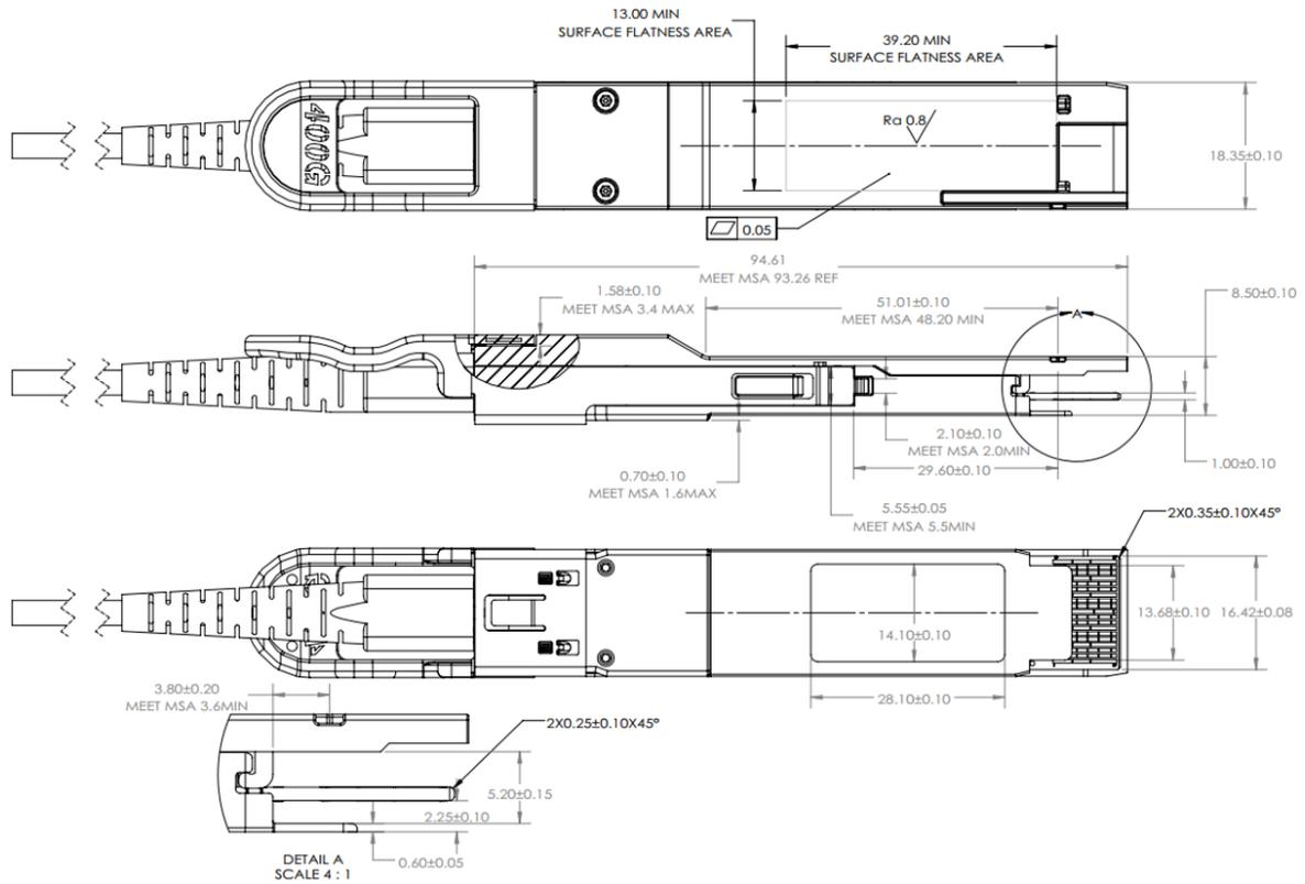
Figure 2. Mechanical Dimensions
