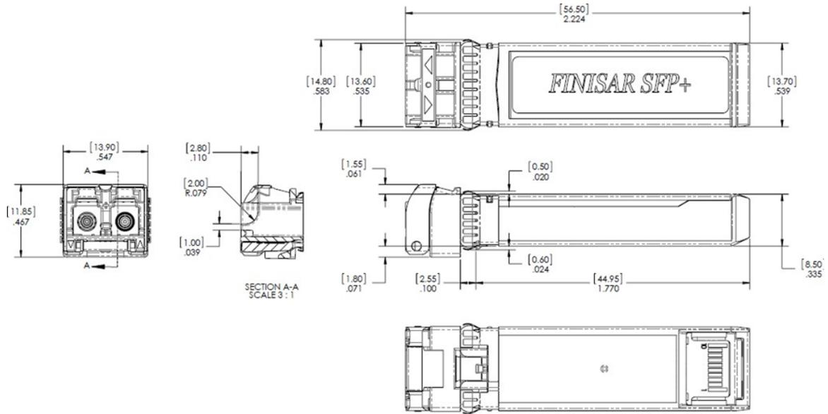
Figure 2. FTLX8574D3BCV Mechanical Dimensions.
