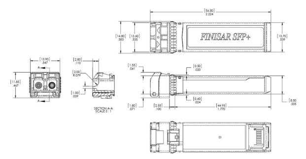
Figure 2. FTLX8574D3BCL Mechanical Dimensions.
