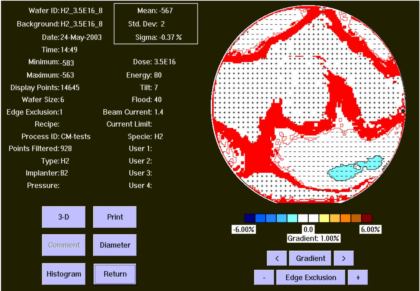
Fig 5 H<sub>2</sub><sup>+</sup>, 80 kV, 7.0E16 H/cm<sup>2</sup> (dose sensitivity ~0.9)
