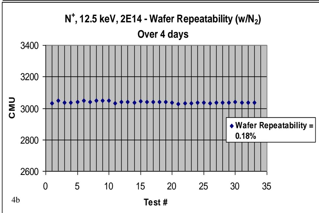
Fig 4a. ULE B repeatability (1.0 keV) Fig 4b. N<sup>+</sup>, 12.5 keV repeatability
