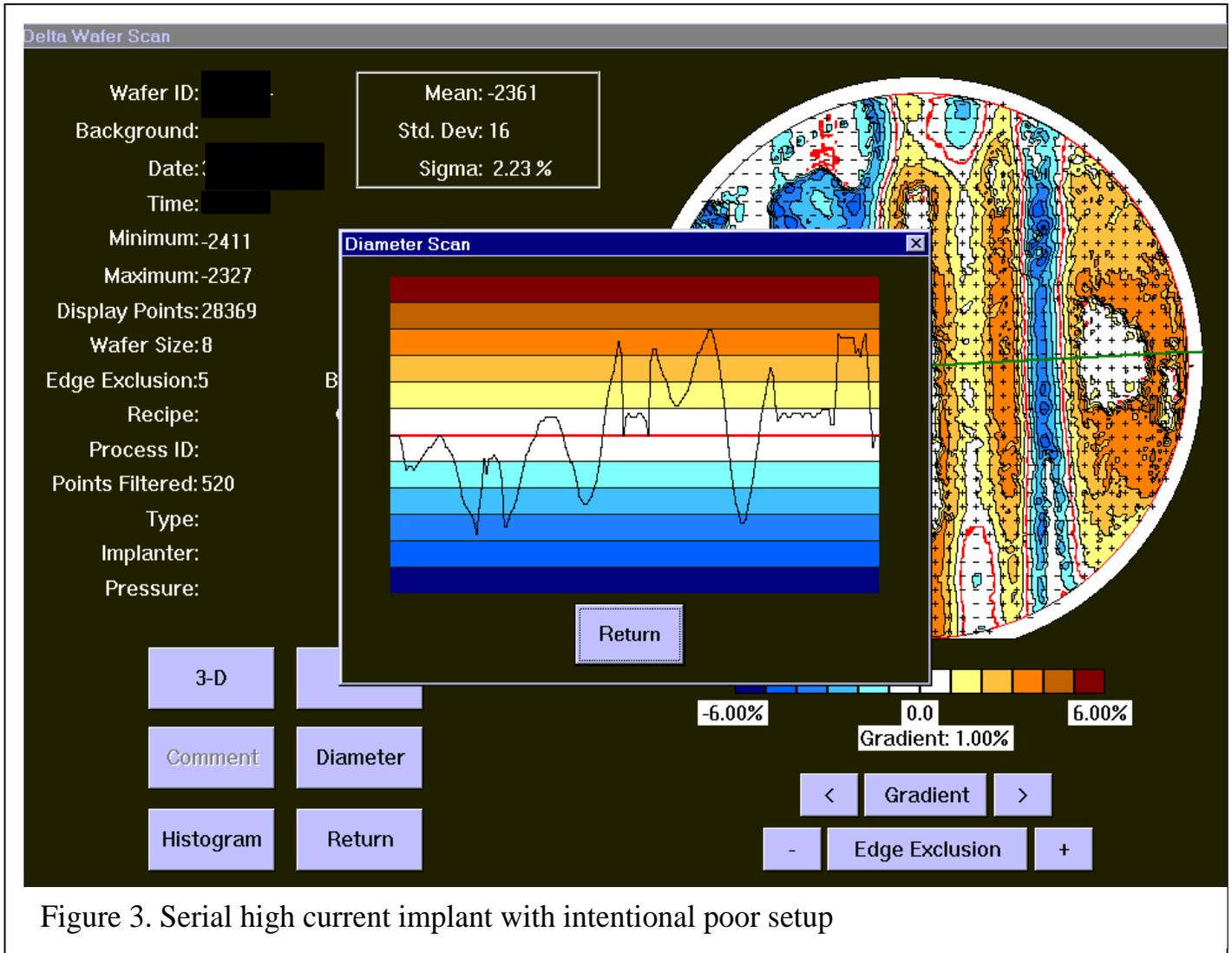
Figure 3. Serial high current implant with intentional poor setup
