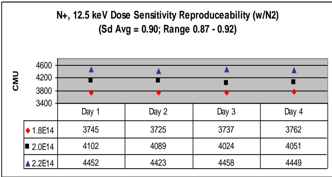
**Fig 2. N<sup>+</sup> dose sensitivity and repeatability of S<sub>d</sub>**
