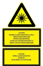
Coherent industrial lasers are designed in strict accordance with the respective safety regulations. We certify that each laser manufactured by our company complies with FDA Radiation Performance Standards, 21 CFR Subchapter J and with IEC 60825. Warning labels as shown in the figure appear on each Coherent laser to indicate the respective classification.
