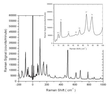
Superior low-frequency Raman spectra can be observed. Sharp, identifiable peaks near 10 cm<sup>-1</sup> are visible in a measurement of L-Cystine.
