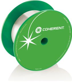
Coherent's Large Mode Area (LMA) Ytterbium-Doped Double Clad Fiber is ideal for high power fiber lasers and amplifiers used in military, industrial, and medical applications. LMA Yb-doped fibers enable efficient, compact, diode pumped fiber sources that are an attractive alternative to traditional solid-state lasers. This fiber features a 10/400 core/cladding size with a low NA (0.075) core, > 77% slope efficiency, > 100W CW output power and is suitable for use in single-mode applications.
