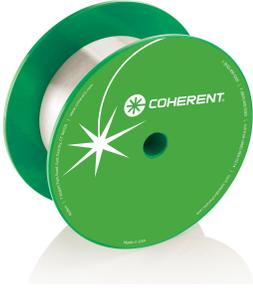
True LMA fiber featuring a unique low NA ( $< 0.1$ ) high concentration Ho-doped core design. The Ho-doped fiber can be pumped by a Tm-doped fiber laser at  $\sim 1950$ -nm and can achieve 60% efficiency. The high NA (0.46) large pump cladding waveguide allows for efficient coupling of high pump powers. The large core diameter (40  $\mu\text{m}$ ) maintains a large mode field diameter and short device length, thereby minimizing non-linear effects such as SBS and SRS.
