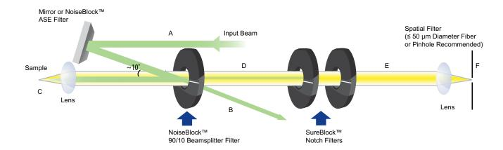
A high throughput, low frequency Raman spectroscopy system can be assembled by combining a NoiseBlock™ 90/10 beamsplitter with two SureBlock™ notch filters and optional NoiseBlock™ ASE suppression filters. The resultant system is capable of measuring Raman signals as low as <10 cm<sup>-1</sup> from the laser line.
