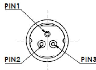
PIN1: Case , PIN2: LD Anode P, IN3: LD Cathode
