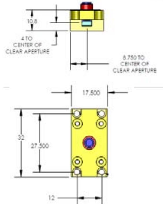
Ondax PicoPulse™ pulse stretcher/compressor filters are produced in a proprietary glass designed for long lifetime, high efficiency and low loss. Ondax's fabrication process is highly stabilized to ensure excellent part-to-part repeatability.
