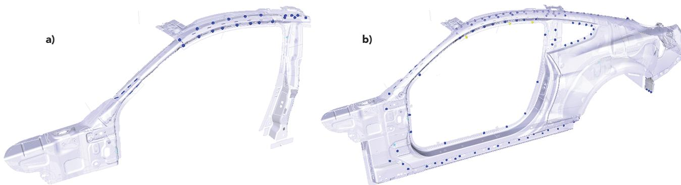
**FIGURE 4.** Structural welds on the body-side inner assembly (a) and body-side outer assembly (b) of the Ford Mustang.
