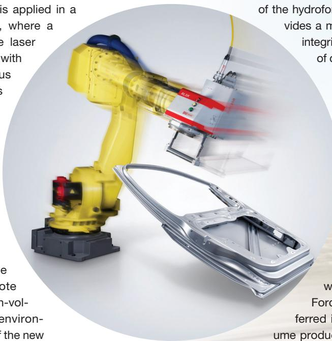
**FIGURE 1. In the Welding-on-Fly mode, the welding head works with a robot in a continuous movement to perform very fast three-dimensional beam positioning.**
