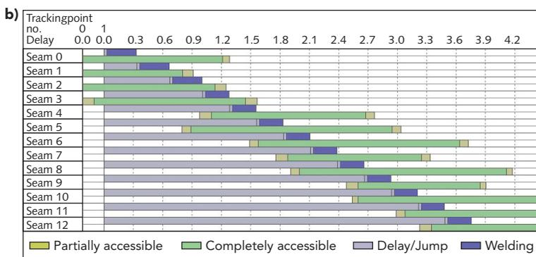
**FIGURE 5.** User-friendly process control using the RLSK Studio software can visualize the focus positioning (a) as well as the welding process in a timeline (b). The timeline shows that there is only a minimal loss of time between the welding of the single seams (shown in blue). Therefore, maximum productivity is achieved. (Portions of [b] were enhanced for readability)
