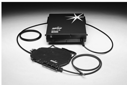
Fig. 5 Small, compact and lightweight fiber amplifiers with remote high power amplifier head have enabled kW level fiber amplifiers to overcome SBS in the delivery fiber and improve their use in the lab for beam combining experiments.
