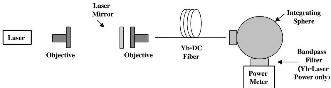
Figure 3 – Schematic of slope efficiency measurement set-up
