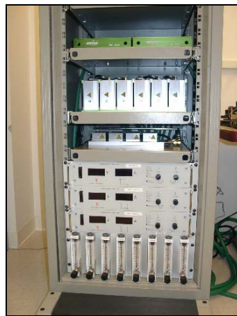
Figure 3: Monolithic LMA fiber including pump diodes and power supplies in a 19" rack mount system.
