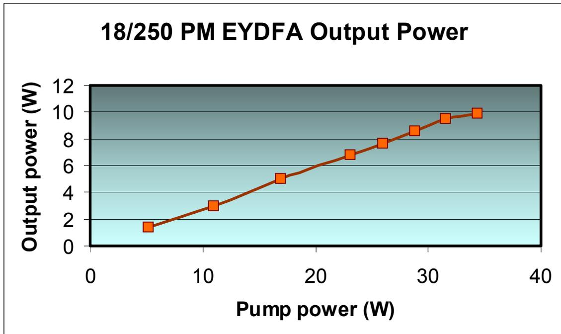
**Figure 2:** Output power versus pump power for the EYDFA.
