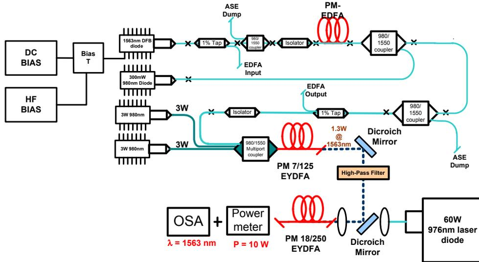
**Figure 1:** Experimental setup of our 10W fiber laser source emitting over 10W at 1563nm.
