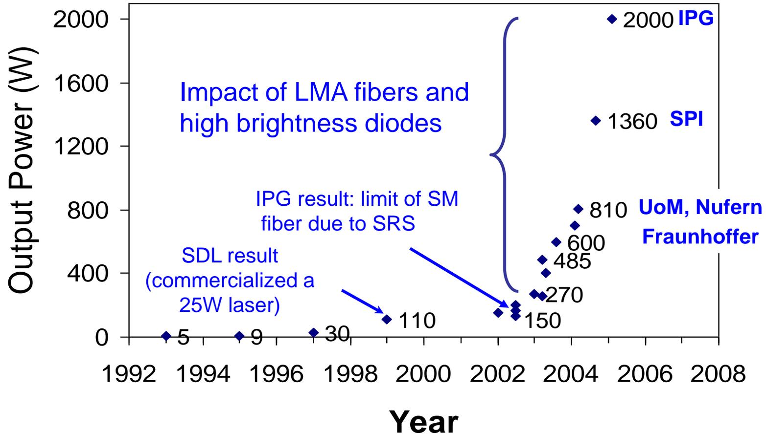
Fiber lasers are a viable alternative to more conventional solid state lasers
