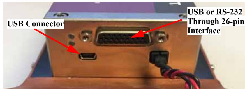
**Figure 4-15. Connectors for a USB or RS-232 Connection**
