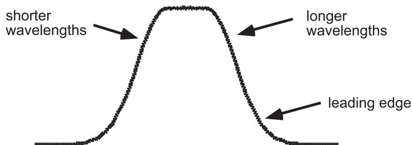
**b. Positive Chirp — Red Frequency Components Lead The Blues
