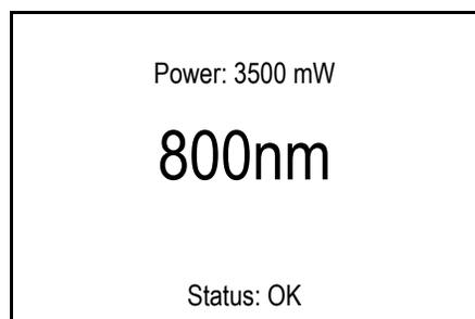
The user must access this menu to adjust the Chameleon Ultra, Vision, or Vision-S output wavelength. Select the desired wavelength using the front panel power knob and press Menu select.
