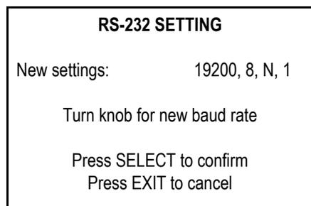
Allows adjustment of the baudrate for the RS-232 communications. Press SELECT to accept the new baudrate value before exiting this screen.
