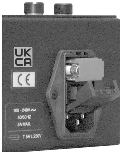
Figure 10-6. Mains Input Showing Fuse Access
