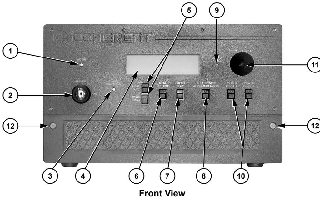
Figure 5-2. Power Supply (Verdi) Ultra and Vision Controls and Indicators
