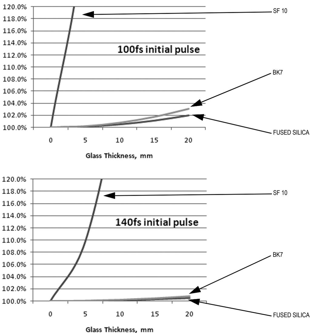
Figure 12-6. Comparison of Pulse Broadening in Fused Silica, BK7, and SF10 (Continued)
