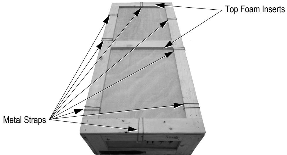
**Figure 11-7. Fitting Top Foam Insert and Clamping the Lid**
