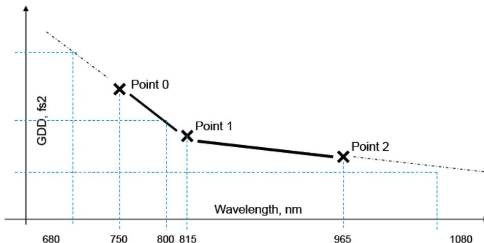
In this example, if a wavelength of 800nm is selected, a GDD value is interpolated from the solid line shown between points 0 and 1. However, if a wavelength outside the defined range is selected, then a GDD value is extrapolated from the last known data for that curve.
