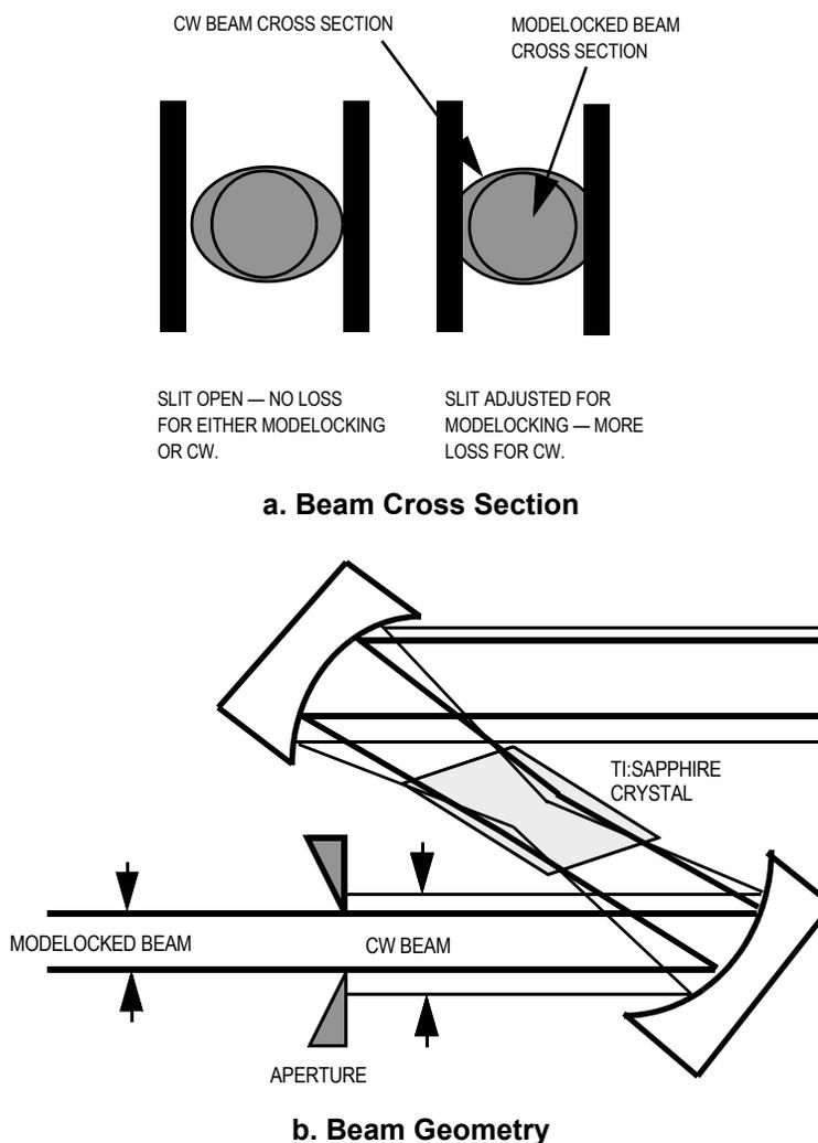
**Figure 12-1. Chameleon™ and Chameleon Vision Saturable Absorber System**
