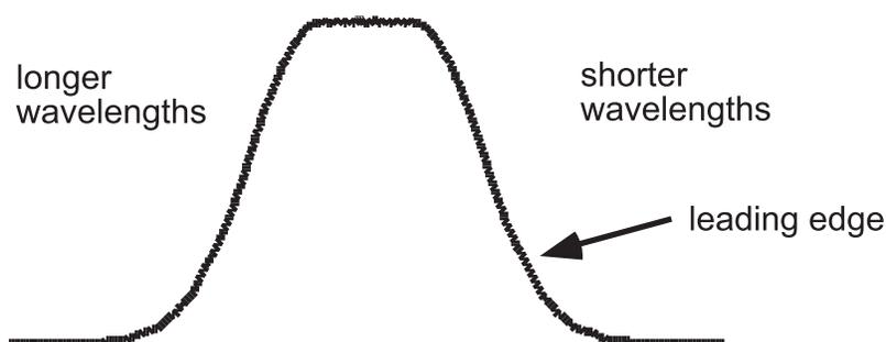
**a. Negative Chirp — Blue Frequency Components Lead The Reds
