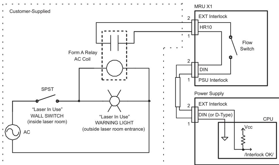
**C. Interlock Circuit Satisfied by Closure of Relay Contacts; Relay Energized by "Laser In Use" SPST Switch**
