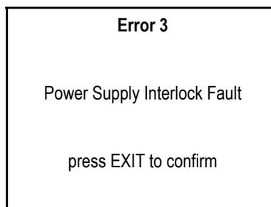
To clear a fault, the appropriate troubleshooting steps should be taken. The power supply keyswitch should be turned to the STANDBY position and the EXIT pushbutton pressed. See Table 8-1, “Troubleshooting/Fault Messages,” on page 85 for a complete listing of system faults and troubleshooting procedures.
