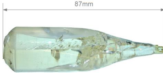
Fig. 2 Yb:CaGdAlO 4 boule after 12 h annealing treatment under reducing atmospheric conditions.
