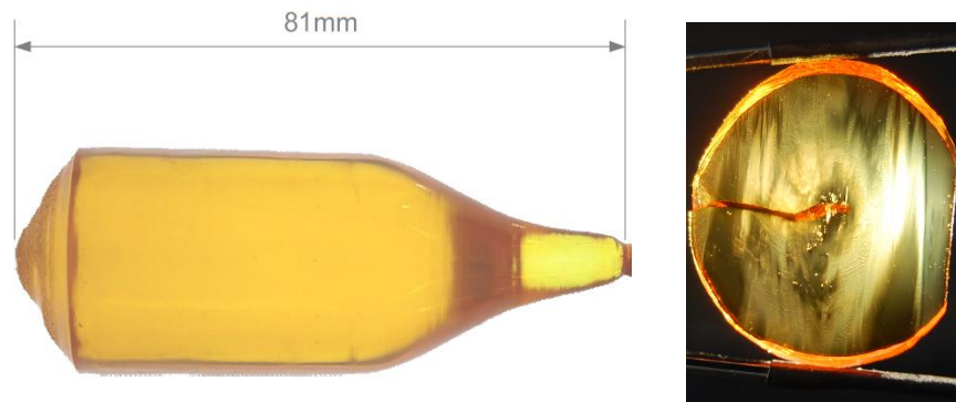
Fig. 1 As-grown Yb:CaGdAlO 4 crystal from 2006 (left). Typical appearance scheme of cloudlike inclusions of 2 μm to 5 μm size (right). Diameter of crystal sample 25 mm.
