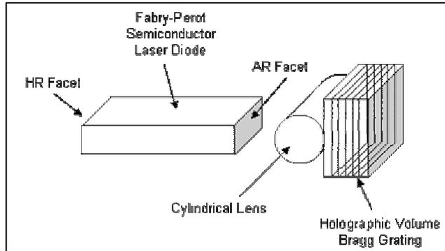
Figure 1. Hybrid ECL/DBR Laser (HECL)
