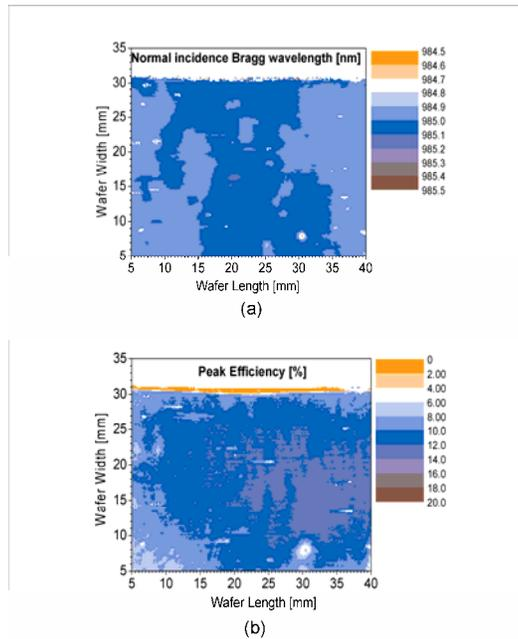
Figure 4. VHG wafer testing: 250  $\mu\text{m}$  resolution measurement across 30 x 40 mm wafer. (a) map of normal incidence Bragg wavelength. (b) Map of peak diffraction efficiency
