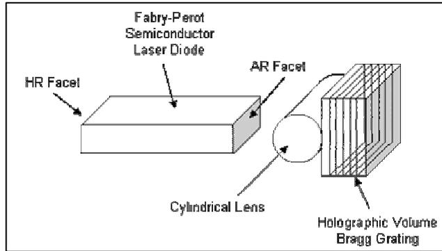
Figure 1. Hybrid ECL/DBR Laser (HECL)
