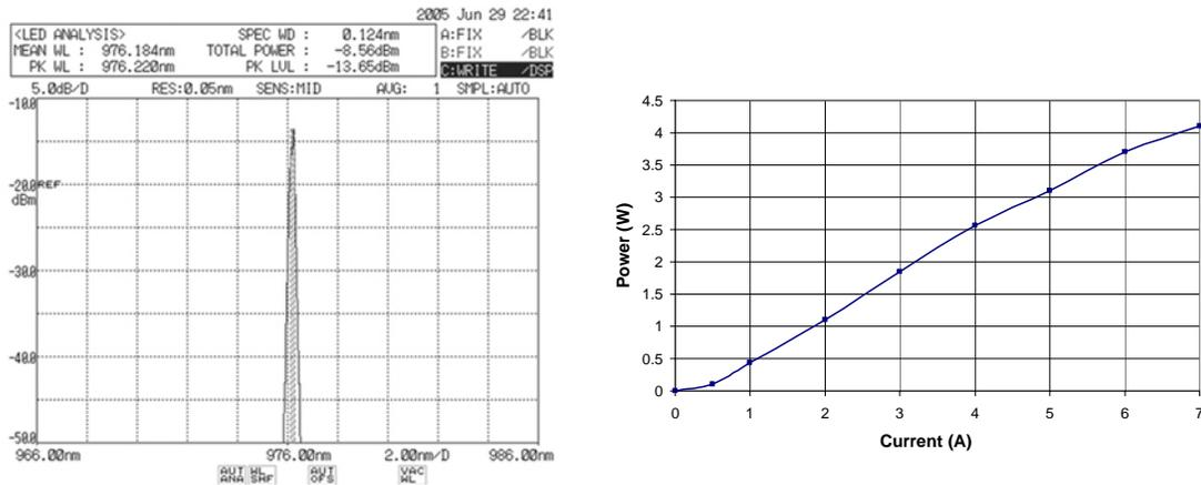
Figure 8. Spectral Plot and LI Curve of High Power/High Spectral Brightness 976 nm Spectrum Stabilized Laser
