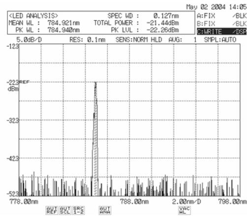
Figure 2b. Spectrum Stabilized Fabry-Perot Laser in HECL Configuration
