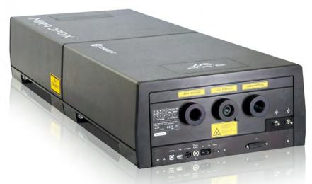
Mira OPO-X is a synchronously pumped, widely tunable, optical parametric oscillator (OPO) accessory that dramatically extends the wavelength coverage of our fs and ps Ti:Sapphire lasers (such as Mira and Chameleon) from 505 nm to 4000 nm. It is fully automated, i.e. software controlled tuning over the full specified wavelength range. This is made possible by its advanced control electronics, built-in diagnostics, and powerful control software package.
