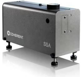
The SSA accessory is designed for use over a broad range of energies and wavelengths. Available in configurations to measure femtosecond or picosecond pulses, this is an accurate and versatile tool compatible with both commercial amplifier systems – Astrella and Legend Elite – and with home-built amplifier systems.
