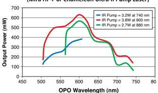
Mira OPO-X (VIS+IR) fs Typical Output Power M (Mira HP-F or Chameleon Ultra-II Pump Laser)
