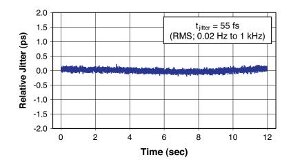
Example showing relative jitter between pulse trains from two synchronized Mira-900 lasers
