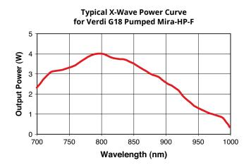
Typical X-Wave Power Curve for Verdi G18 Pumped Mira-HP-P
