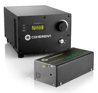
The Verdi G-Series is a revolutionary green pump laser that uses a semiconductor chip as the active medium in place of a conventional laser crystal. This chip has a thickness of only a few microns and is pumped by a diode laser, to generate an infrared beam at a wavelength determined by the chip properties. In all the Verdi G models, the oscillating wavelength is 1064 nm intracavity doubled to produce a 532 nm green output beam.
