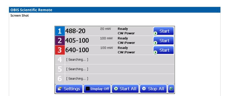
**Figure 1:** OBIS LX/LS Scientific Remote for up to six lasers. Lasers sold separately.
