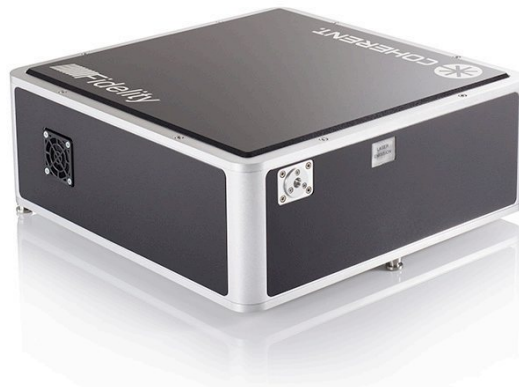
Figure 1. Fidelity-2 is a compact, sealed industrial-grade laser that provides over 2 watts of output power at 1070 nm with a pulsewidth < 55fs.
