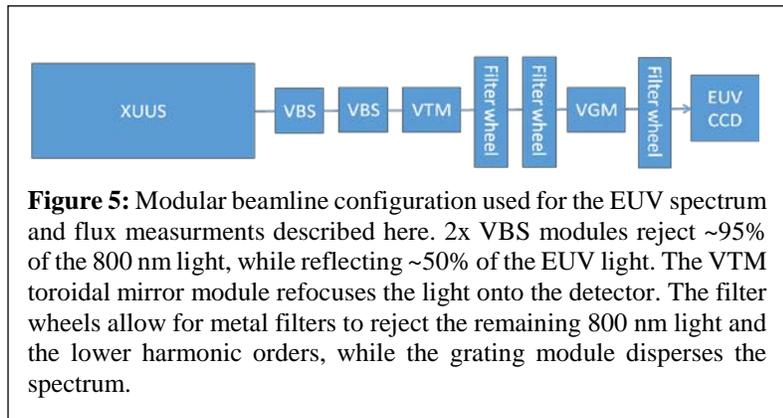
range of the detector, but outside range of wavelengths that are spectrally resolved. KMLabs has developed rigorous procedures that protect against false measurements. In the most rigorous process, the aggregate flux in an HHG beam is measured using a NIST-calibrated photodiode, with the spectrum subsequently dispersed onto a CCD to allow for the flux per harmonic order to be determined.
