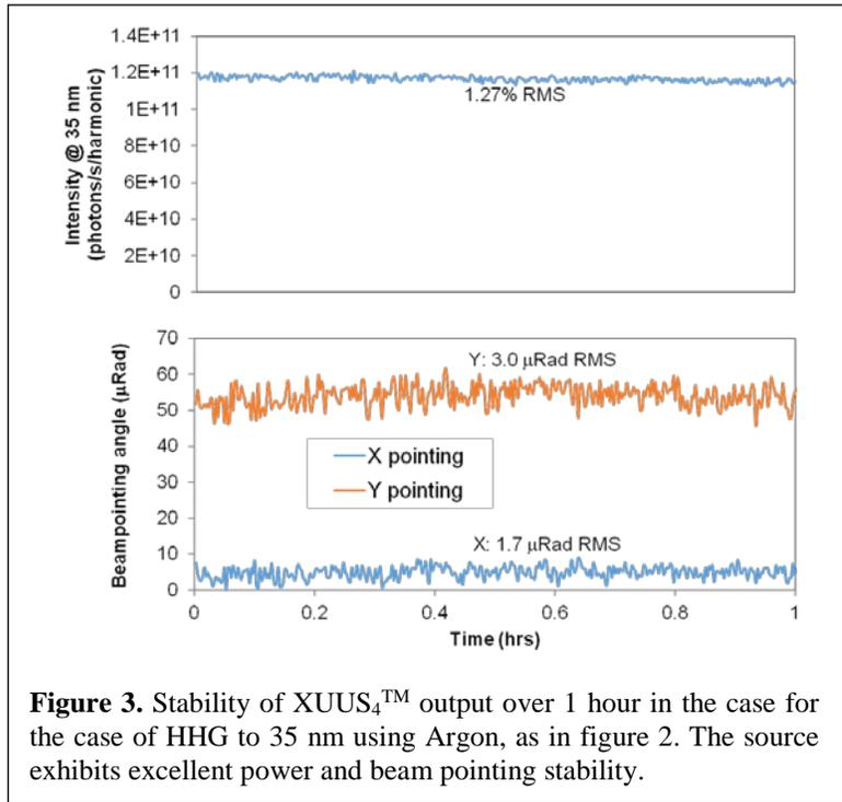
**Figure 3.** Stability of XUUS<sub>4</sub><sup>™</sup> output over 1 hour in the case for the case of HHG to 35 nm using Argon, as in figure 2. The source exhibits excellent power and beam pointing stability.
