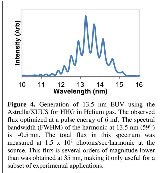
**Figure 4.** Generation of 13.5 nm EUV using the Astrella/XUUS for HHG in Helium gas. The observed flux optimized at a pulse energy of 6 mJ. The spectral bandwidth (FWHM) of the harmonic at 13.5 nm (59<sup>th</sup>) is  $\sim 0.5$  nm. The total flux in this spectrum was measured at  $1.5 \times 10^7$  photons/sec/harmonic at the source. This flux is several orders of magnitude lower than was obtained at 35 nm, making it only useful for a subset of experimental applications.
