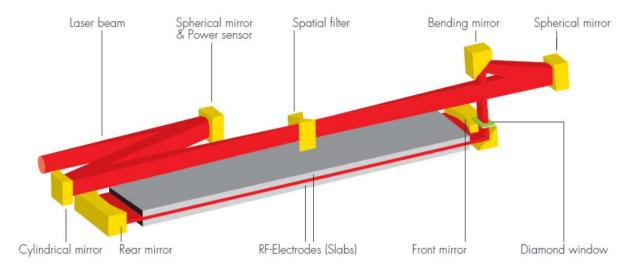
*Figure 3.* In a slab discharge laser such as the Coherent DC 030, the laser gas is RF excited by two closely spaced flat electrodes. The laser power scales with the area of these electrodes.
