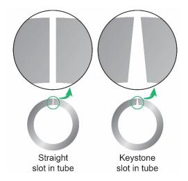
*Figure 4. Slots with a keystone cross section are designed to eliminate blocking with trapped particulates. These slots are particularly difficult to create with non-laser methods.*
