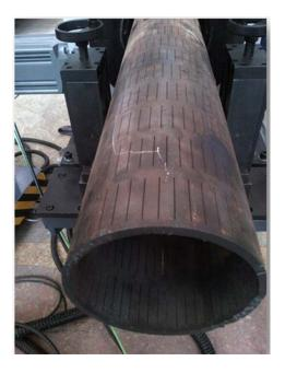
*Figure 1. Slotted liners used for heavy oil production incorporate thousands of slots that must be cut to specification.*
