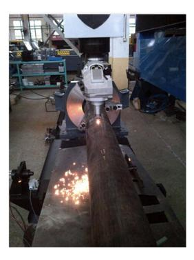
*Figure 2. This application requires a multi-kilowatt laser to achieve target throughput rates.*
